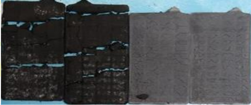
Positive plate was decayed
