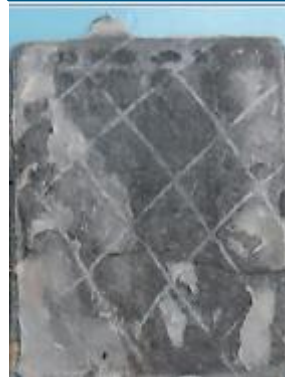
Negative plate sulfated
